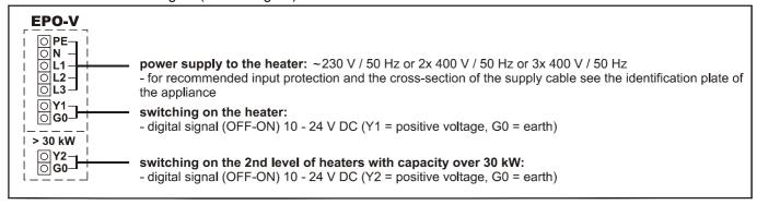
When the electric heater is used together with a DUPLEXVENT unit with built-in control, this control ensures that all conditions for the safe operation of the heater are met.
